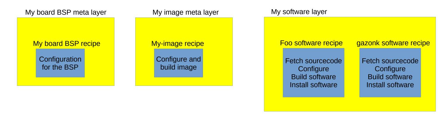
• To build the software for different boards we swith the BSP layer.
