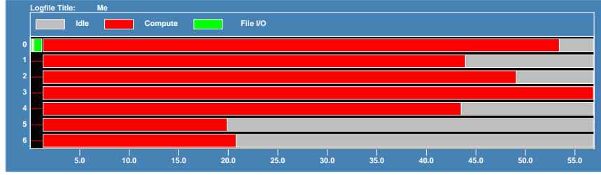
Figure 9.5 Snapshot with nupshot utility of static load distribution, N = 7 .
