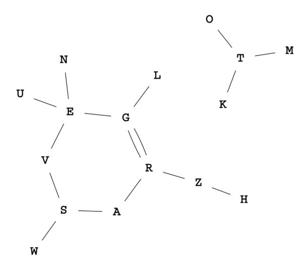
The aim is to have one connected graph with as many loops as possible. If a menu does not contain enough letters and/or loops there will be many false stops of the Bombe meaning that there will be a lot of work until we can determine the correct key.
