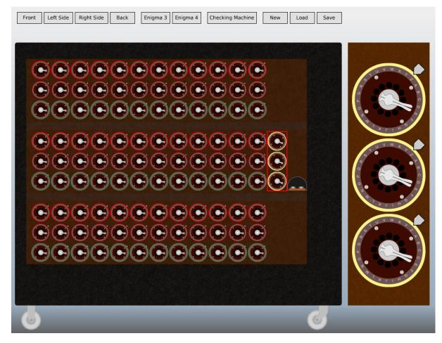
First we select which set of rotors we will try and in which order. Since we use no more than 12 drum banks we can try three rotor orders at once if we wish. However, for now we will just try one order; II, V, III, which happens to be the correct one.
