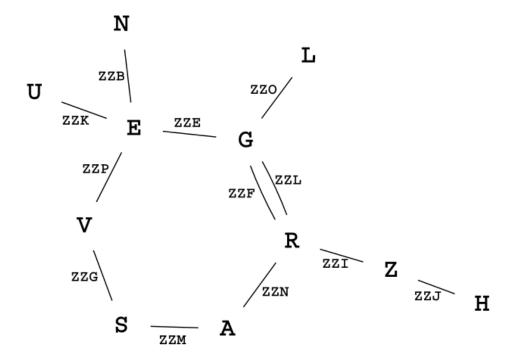
Assign a drum bank to each link in the graph and write the number of the drum bank in a table together with the assumed rotor position. Try to get a continuous sequence of drum banks following the flow of the graph. This simplifies the way the wires are connected on the back of the Bombe by allowing us to use special bridge connectors that connect the output of one drum bank to the input of the very next one.
